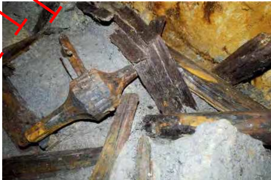
Waterwheel hub – still in connection with its spokes – discovered in Cătălina Monulești Mine. Two complex treadmill-powered water-dipping wheel systems (Cătălina Monulești, and Păru Carpeni mines) were found installed in multiple chambers, one upon the other, and which eventually discharged via a short adit. (© C. Tămaș)
